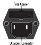
The fuse is located in a slide-in carrier which also contains a spare fuse. The fuse carrier can only be pulled out after the IEC power cord is unplugged. When the carrier is opened the first fuse to be seen is the spare fuse. Remove and safely dispose of the fuse with the blown link before replacing it.
