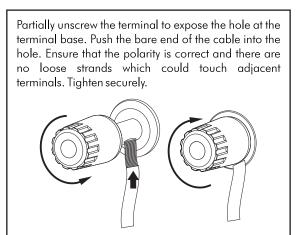
Quad Platinum power amplifiers use two sets of loudspeaker connectors per channel. The positive and negative terminals of each channel are internally connected. If you are single wiring your loudspeakers (for example to a pair of Quad Electrostatics) you may use either pair. If you are bi-wiring your loudspeakers with two sets of cables, you may find it more convenient to use both sets of terminals. The wiring diagrams on the next pages will help you.
