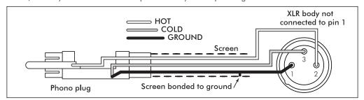
The important point is that the 'cold' line is connected to ground at the remote (phono) end, and not at the XLR. Thus the balanced inputs at Pins 2 and 3 see only the voltage at the phono plug itself, and any spurious voltages that may exist on the ground line are ignored.
