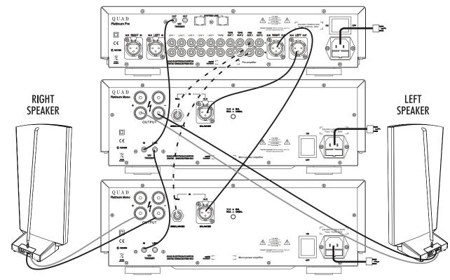
Platinum Mono Amplifiers with Loudspeaker Bi-Wiring
