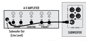
Alternatively, you may use a split mono lead from the processor to both inputs of the subwoofer. In this case the input level at the subwoofer will be slightly higher.
